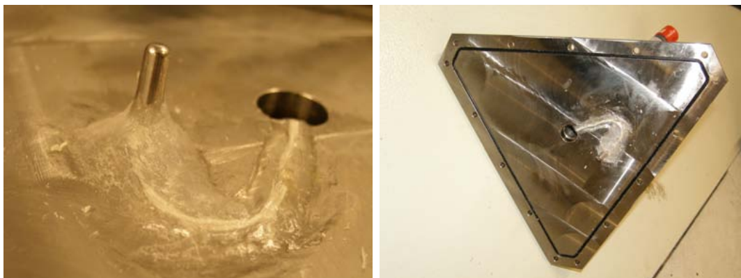
Figure V.7: The PT100 sensor glued to a cooling plate; the wire is passed through a former water outlet.
