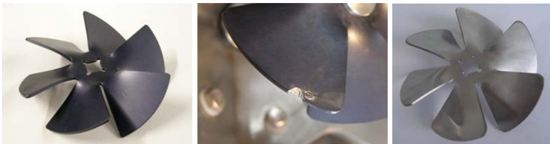
Figure V.3: figure on the left: propeller made out of anodized aluminum, the diameter is 10 cm;
